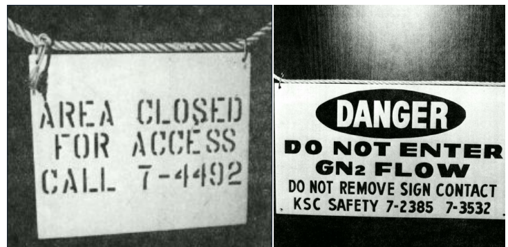
Figure 4: Access control signs (left) can be removed without concurrence from Safety Personnel. After the accident, personnel were required to use the sign depicted at right for GN 2 purges.
