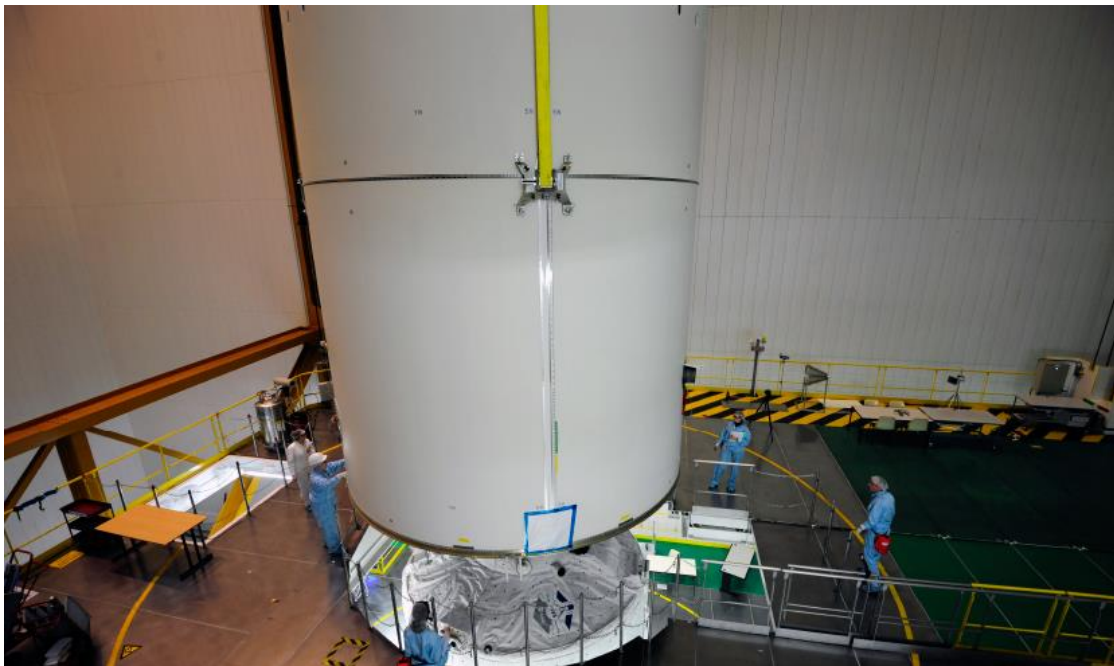
Installing the fairing on the ATV-5 © ESA
