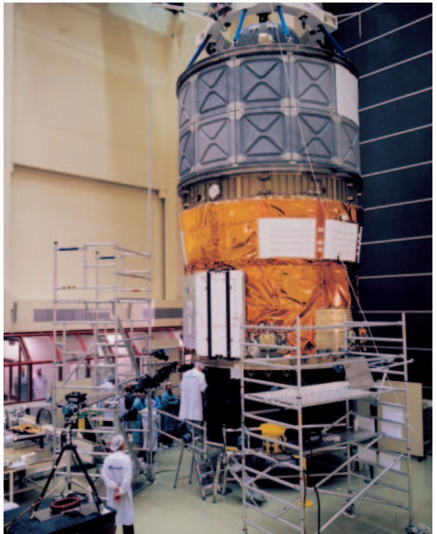
Figure 9. ATV shock test set-up in the HYDRA preparation area
