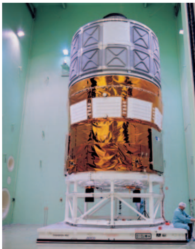
Figure 4. ATV on the Acoustic Stand in LEAF
