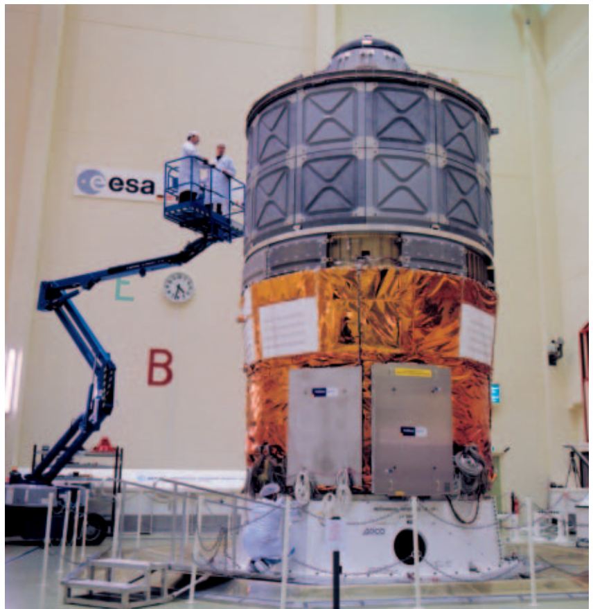
Figure 6. Longitudinal modal survey test set-up on HYDRA
